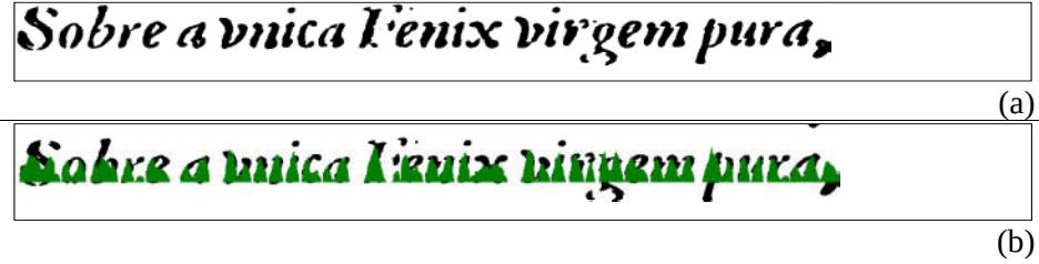
Fig. 6. Word detection: (a) input line and (b) superimposed projection profile
